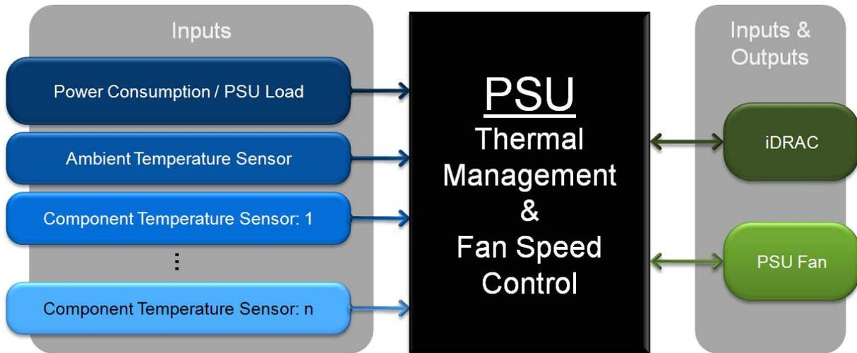
**Figure 8. Inputs and Outputs of PSU Thermal Management**
